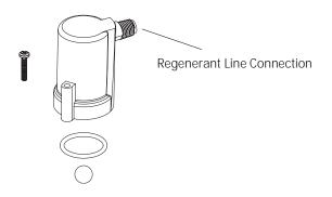
Figure 11 Regenerant Connection for Performa Valve
