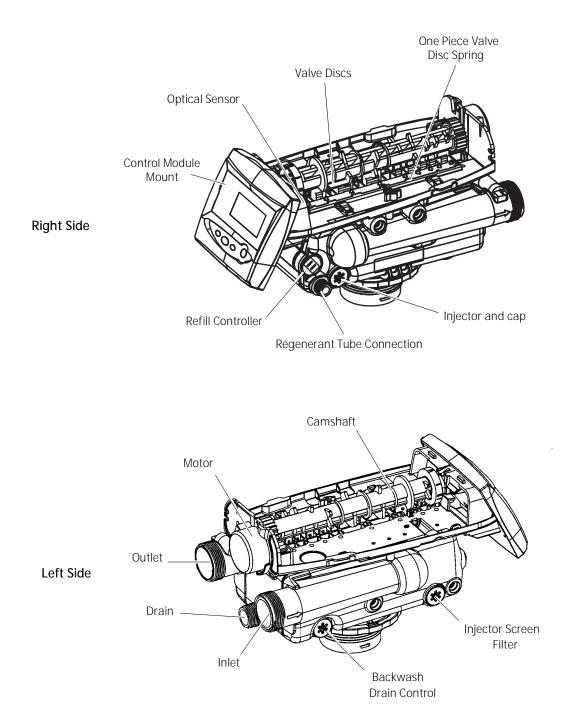
Figure 4 700 Series Controller Identification
