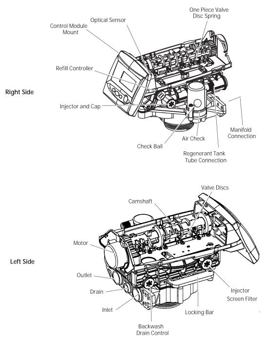
Figure 3 Performa Valve Identification
