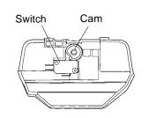
This microswitch is mounted behind the controller at the front end of the camshaft. The switch is mounted to the top plate. The cam for this switch is screwed to the front of the camshaft. This cam can be adjusted to activate the microswitch at any time during the regeneration cycle.
