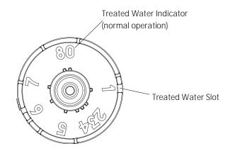
The corresponding slot for the number is positioned at the optical sensor which is approximately 90 degrees out of phase.
