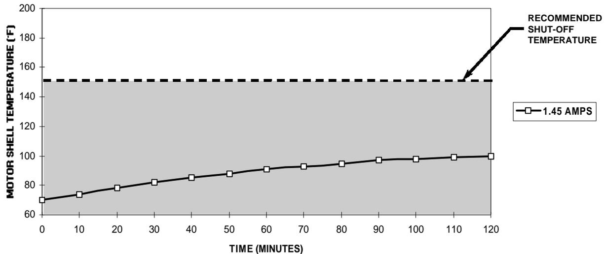
All of the pump models in the Performance Data and Heat Rise charts are in the shaded area, meaning they are capable of sustaining continual running, at any of the above listed pressures, without shutting down to allow the motor to cool. To conserve wearing parts, however, the pump should only operate as needed.
